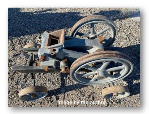
What a cool thing this is! This is Bill Lanier's rock crusher. It ran all day. Hook up a flat belt from an engine and around the flywheel. The flywheels go round and round. If you look down in the hopper you can see the jaw crushing rocks. Assayers used this to crush miners samples to evaluate them according to Bill. For some reason, this reporter was fascinated by this machine.
